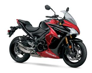
For riders who desire a full fairing on their street sportbike, Suzuki also offers the 2016 GSX-S1000F ABS, which takes the performance of the GSX-S1000 and adds a fairing, a short windscreen, a dual-headlight face, and Suzuki's digital Antilock Brake System (ABS) that monitors wheel speed and matches stopping power to available traction.
